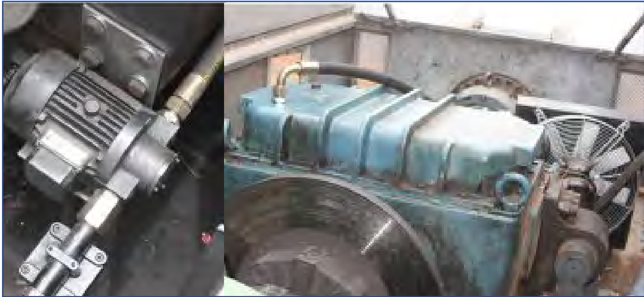
Gear Oil Cooler with Air Ventilator and Increased Radiated Air fins
