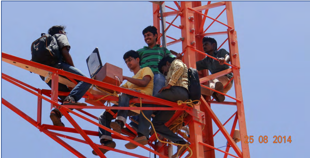
Photonic system validated with the 120m met mast and other remote sensing instruments results at Kayathar
