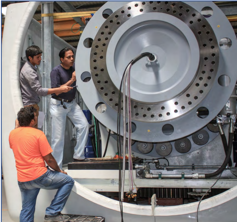
Factory Instrumentation of Garuda 1700 kW WT
